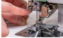
Needle Threading System
