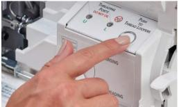
RevolutionAir™ Looper Threading Insert thread into one of the Acclaim's threading ports, push the button and a gust of air quickly pushes it through the patented tubular loopers, exactly where you need it every time. Tangles, knots and breakage are now a thing of the past!
